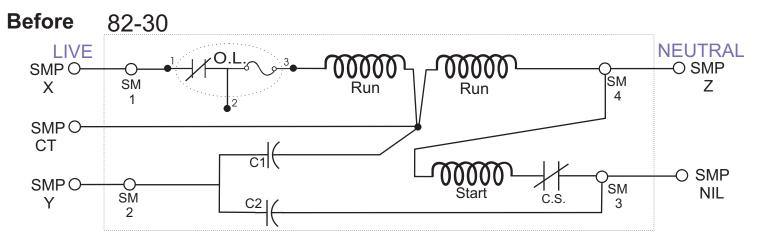
The RED and BLUE wires of the Solid State Start Switch take the place of the mechanical start switch.
